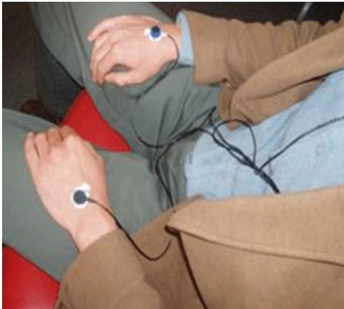
The Qline assessment consists of two sections: a stress measurement and a vitality (fitness) measurement. These measurements are made by recording a series of heartbeats, and registering every heartbeat interval. This series of intervals forms a data set on which the analyses are largely based. For the measurements themselves is done with three sensors that are placed on the body and are wirelessly connected to a computer.
